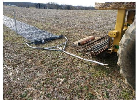
The crew spent less than \$250 to purchase new hydraulic hoses, steel, and hardware. The rest of the materials were scrap or items on hand. The device helps the crew safely and efficiently install temporary snow fence in about one-third the time of previous years. Three workers can install approximately 2,500 feet of snow fence in roughly seven hours.
