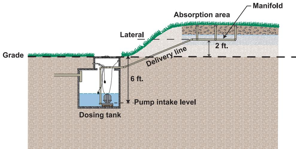
Elevation change from pump intake to grade = 6 ft.
