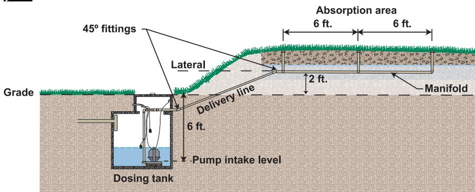
Add the lengths of all the sections of pipe from the pump to the manifold, including the manifold. Do not include the lateral pipes; the head loss due to friction in the laterals is assumed to be 0.
